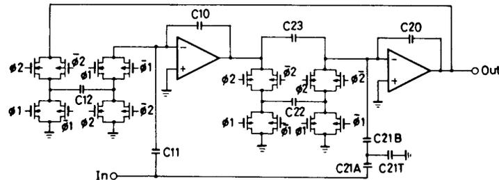
Fig. 4 Schematic of 46.20 kHz band-pass filter
