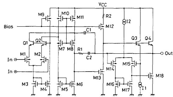
Fig. 5 Operational amplifier used in filter blocks
