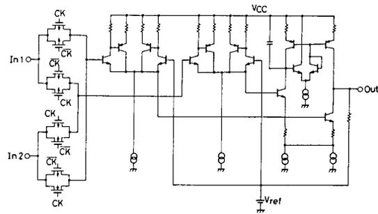
Fig. 3 Subtracter section
