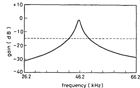
Fig. 8 Frequency response of the 46.20 kHz band-pass filter
