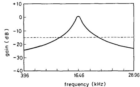
Fig. 7 Frequency response of the 16.4 kHz band-pass filter
