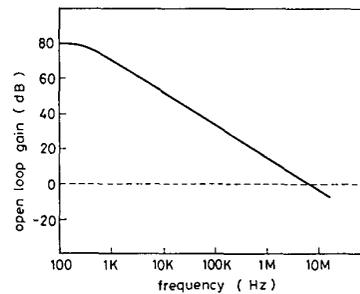
Fig. 6 Frequency characteristics of the operational amplifier in filter blocks
