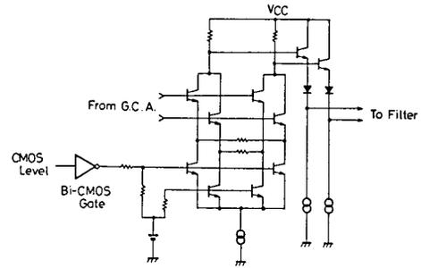
Fig. 2 Interface scheme between CMOS and analog in the balanced demodulator section
