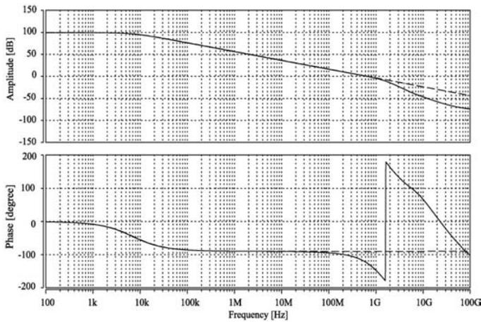
Fig. 4. The gain and phase frequency characteristics (dotted: equivalent circuit model from reference 3, solid: SPICE simulation result of the circuit in Figure 3).
