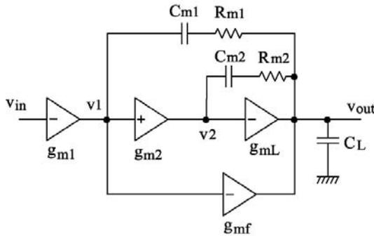
Fig. 1. Nested mirror compensation with feedforward gm stage and nulling resistors.
