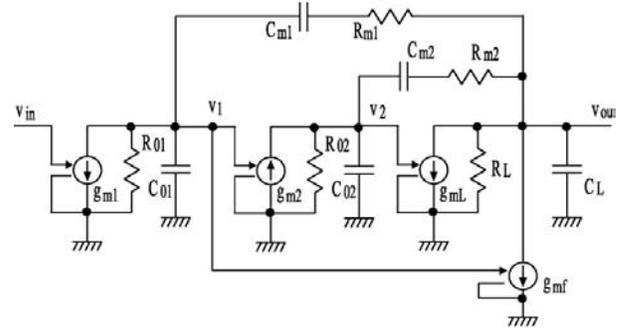
Fig. 2. The small-signal equivalent circuit of the circuit in Figure 1 with stray capacitors.
