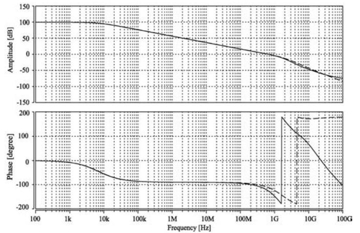
Fig. 5. The gain and phase frequency characteristics (dotted: equivalent circuit model in Figure 2, solid: SPICE simulation result of the circuit in Figure 3).
