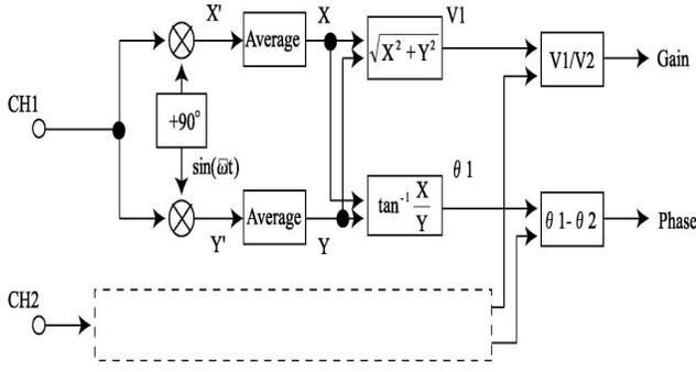
Fig. 4. Calculation of the loop gain and phase at a frequency of  $\omega$ .
