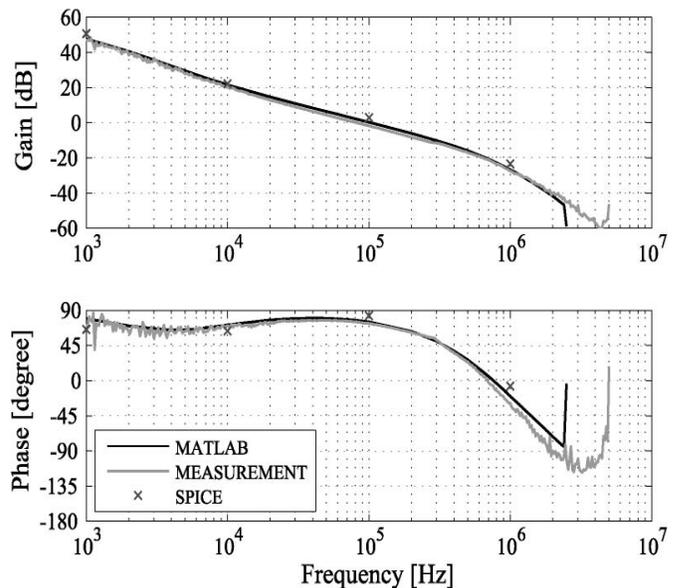
(c) Gain and phase of the total loop ( $V_{in}=2.5V$ ;  $V_{out}=1.5V$ ).
