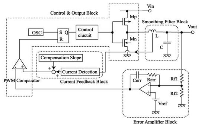
Fig. 1. Block diagram of a current-mode buck DC-DC converter.
