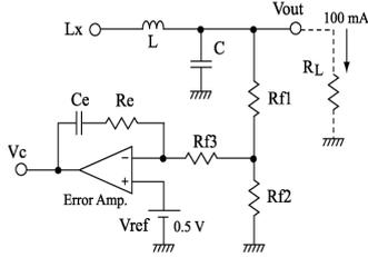
Fig. 6. The circuit configuration in the voltage feedback loop.
