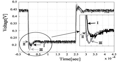
(b) The transient response at the error amplifier output.
