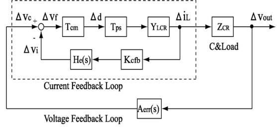
Fig. 3. The small signal equivalent circuit of a DC-DC converter in Fig. 1.
