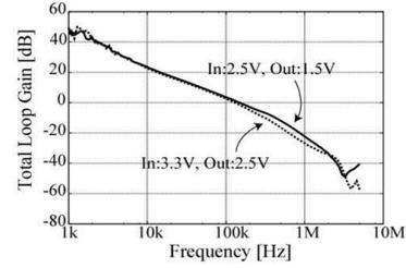
(a) Gain characteristics: 0 dB bandwidths are 150 kHz and 136 kHz.
