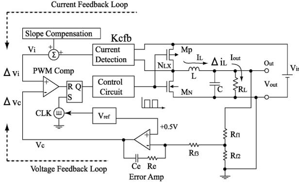
Fig. 1. Block diagram of a designed MOS current-mode buck DC-DC converter.
