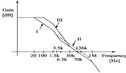
Fig. 7. Frequency characteristics of the total feedback loop for various configurations in an error amplifier.
