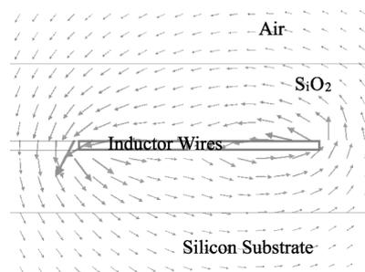
Figure 1. Direction and strength of the magnetic field vector around the inductor wires.
