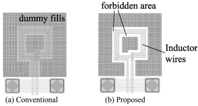
Figure 3. Layout patterns of examined on-chip spiral inductors.
