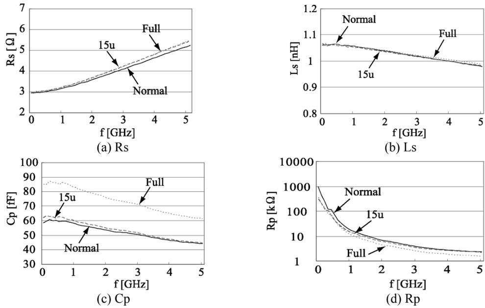
Figure 5. Measured frequency characteristics of parameters in the equivalent pi circuit model with and without metal dummy fills.
