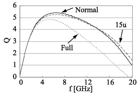
Figure 4. Measured Q-value frequency characteristics with and without metal dummy fills.
