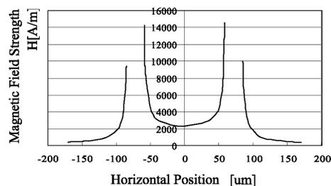
Figure 2. Magnetic field strength around the inductor.
