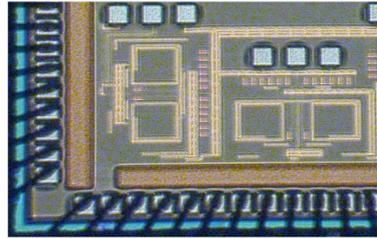
Fig. 7 Chip microphotograph of the pMOS-type (left) and ref-type (right) VCOs.
