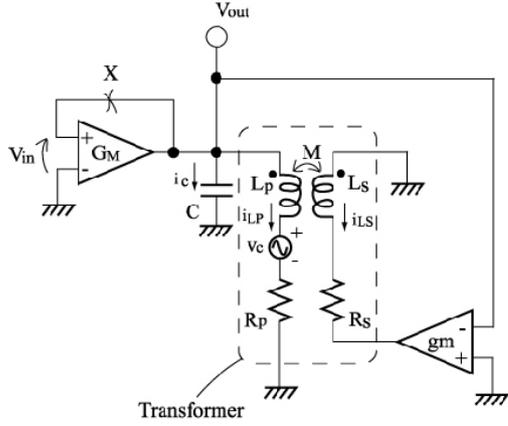
Fig. 2 The Q-value enhancement circuit having the external feedback path.
