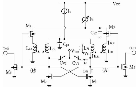
Fig. 4 Schematic of the Q-value enhancement VCO circuit.
