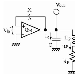
Fig. 1 Conventional LC oscillator circuit.
