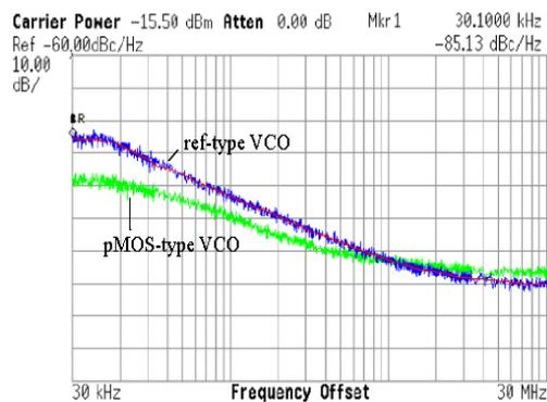
Fig. 6 Phase noise comparison.
