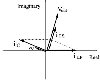
Fig. 3 Phase relationship of voltages and currents in Fig. 2.
