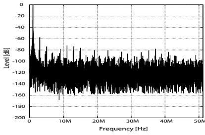
Fig. 5. The frequency spectrum of the simulated conventional 14-bit ADC.
