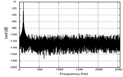
Fig. 8. The frequency spectrum of the simulated 14-bit ADC in Figure 4.
