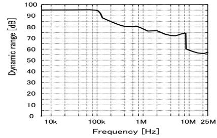
Fig. 7. The input signal frequency vs. SFDR characteristics of the ADC in Figure 3.
