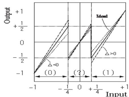
Fig. 1. The input vs. output voltage relationship of a 1.5-bit bit-block.
