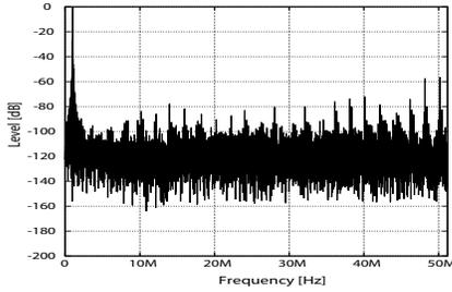
Fig. 6. The frequency spectrum of the simulated 14-bit ADC with permuting capacitors.
