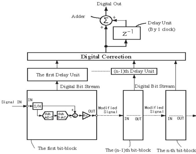
Fig. 3. Block diagram of the proposed ADC with 1.5-bit bit-blocks and an averaging function at the output.
