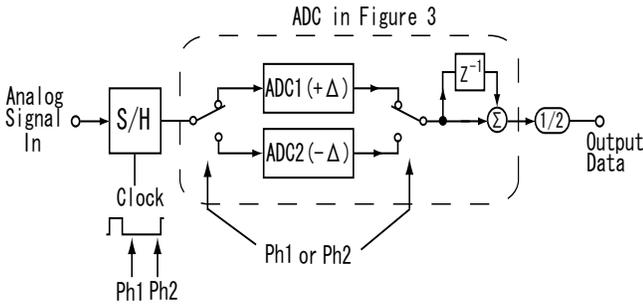
Fig. 4. The ADC with a sample-and-hold function in front of the ADC in Figure 3.
