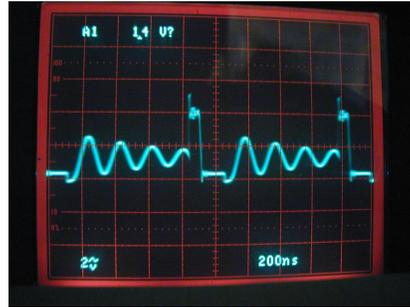
Fig. 9: Waveform at the out terminal in light-load mode
