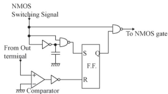
(a) Light-load mode control circuit
