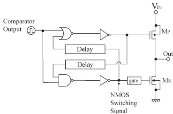
Fig. 4: Pulse control and output circuit
