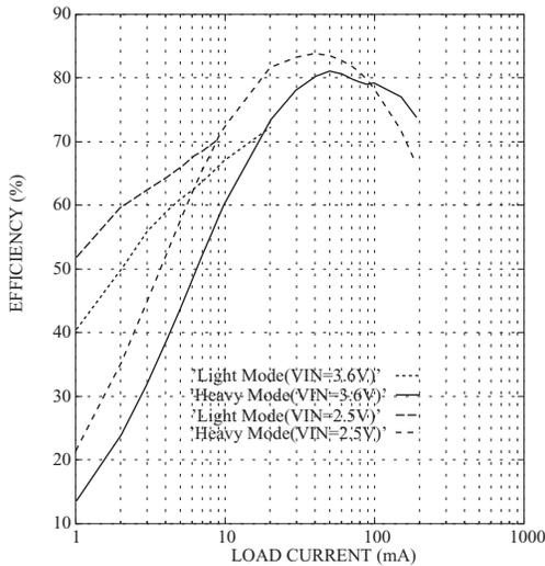
Fig. 6: Load current vs. power efficiency
