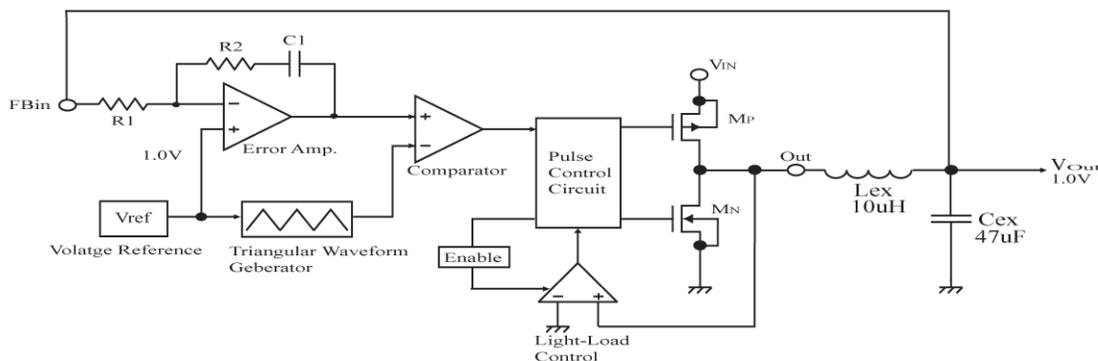
Fig. 1: Block diagram of the newly designed DC/DC Converter
