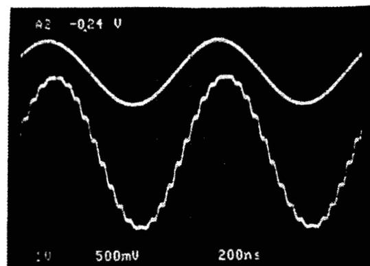
Figure 5. Input and output waveforms (  $f_{in}=1$  MHz, 0 dB full scale input,  $V_{cc}=1.5$  V, clock=20 MHz )
