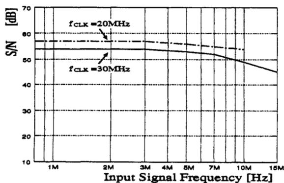
Figure 8. Input signal frequency vs. S/N (0 dB full scale input,  $V_{cc}=1.5$  V)
