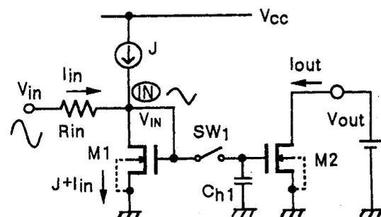
Figure 1. Conventional low-voltage sample-and-hold circuit
