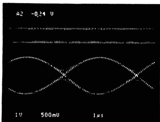
Fig. 6 Result of the beat frequency test (upper, In; lower, out;  $f_{in}=9.9$  MHz, 0dB of full scale;  $V_{cc}=1.5$  V; clock=20 MHz)
