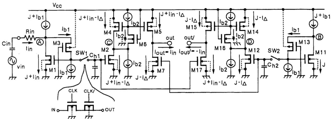
Figure 4. Low-voltage, high-performance sample-and-hold circuit
