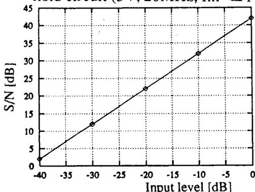
Fig. 5 S/N vs. input signal level (3V, 20MHz,  $f_{in} = 1MHz$ , full scale=0dB)
