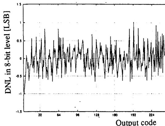
Fig. 7 Differential nonlinearity of an ADC
