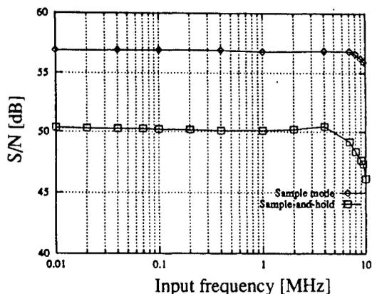
Fig. 4 S/N vs. input frequency of a sample-and-hold circuit (3V, 20MHz,  $I_{in} = \pm 110 \mu A$ )
