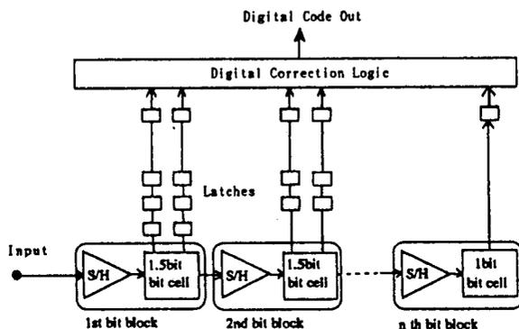
Fig. 1 New pipe-lined ADC architecture
