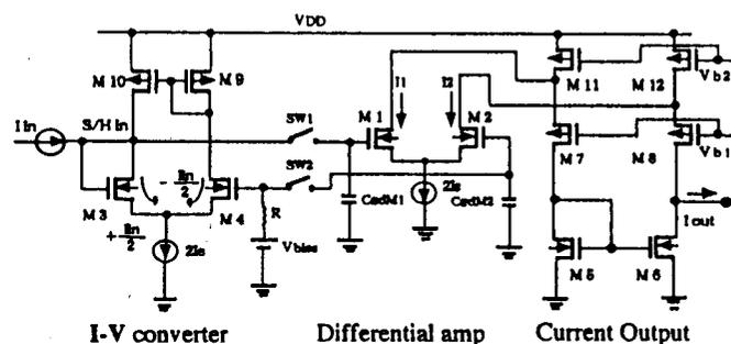
Fig. 2 Schematic of a sample-and-hold circuit
