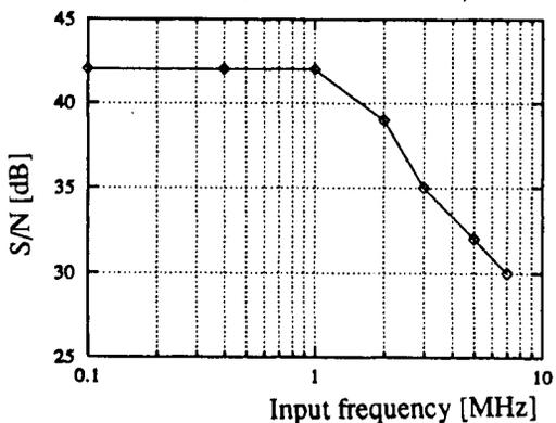
Fig. 6 S/N vs. input signal frequency (3V, 20MHz, full scale input)
