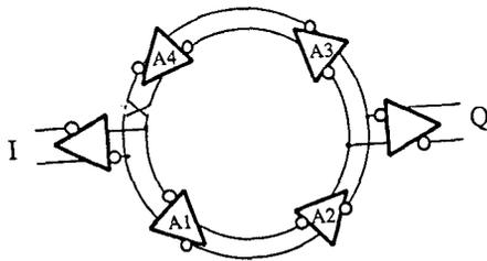
Fig. 2 Generation of I/Q outputs in a ring-oscillator type VCO
