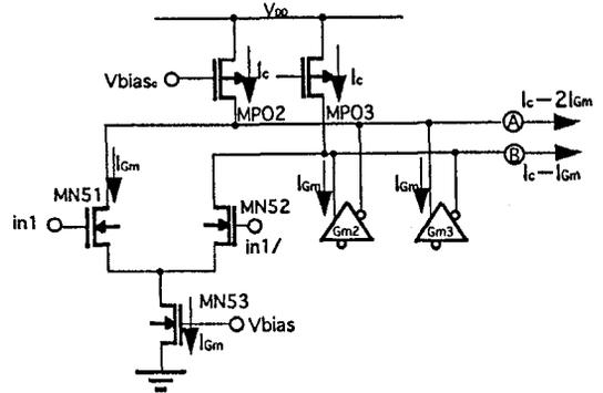
Fig. 7 The gm cell circuit and a current composing scheme
