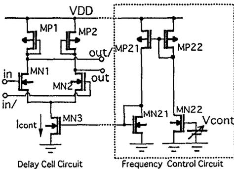
Fig. 6 The delay cell and control circuits
