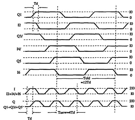
Fig. 5 Waveforms of the circuit in Fig. 4 at different places
