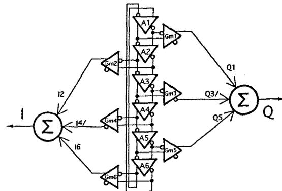
Fig. 4 The new configuration that realizes both high-frequency oscillation and generation of I/Q outputs
