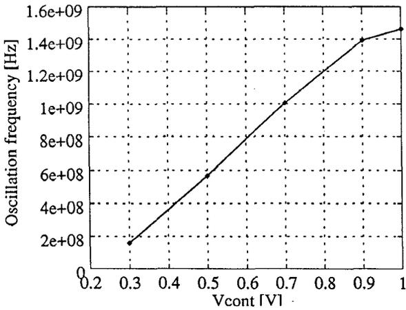
Fig. 9 VCO oscillation frequency versus control voltage characteristic
