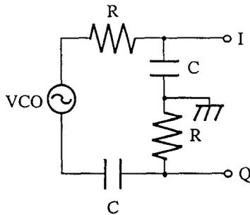
Fig. 1 Conventional RC phase shifter circuit
