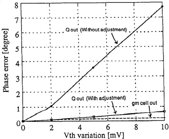
Fig. 11 Phase error at Q output with Vth variation relative to I output
