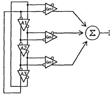
Fig. 3 The configuration that enables high-frequency oscillation
