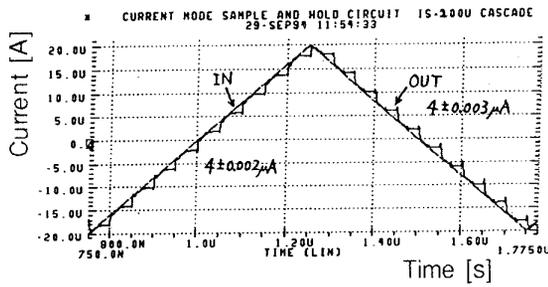
Fig. 7 Input and output current waveforms (Vdd=3V, lin=1MHz, Clock=20MHz)
