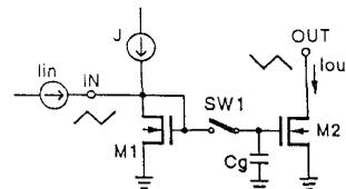
Fig. 3 Basic current memory cell No.2
