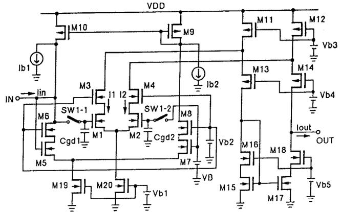
Fig. 6 Sample and hold circuit
