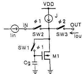
Fig. 1 Basic current memory cell No.1
