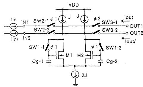
Fig. 2 Differential current memory cell
