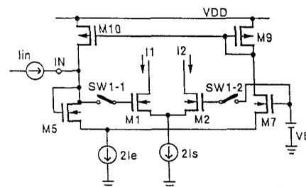
Fig. 4 New differential current memory cell
