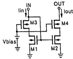
Fig. 5 Current mirror with increased output impedance
