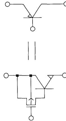
Fig. 1. Basic equivalent high-speed p-n-p transistor configuration.
