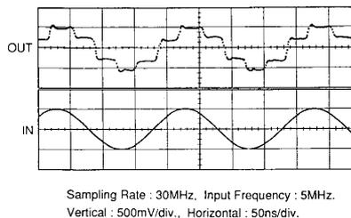
Fig. 8. Typical input and output waveforms for the sample-and-hold.
