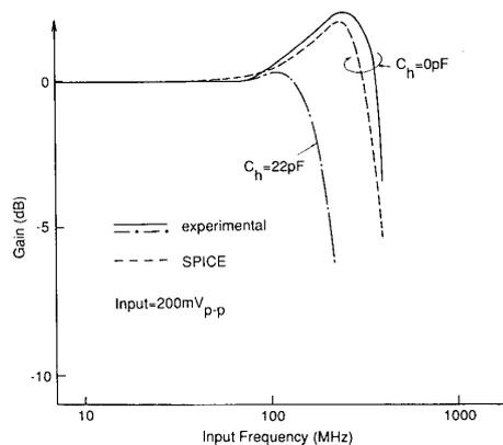
Fig. 7. Frequency responses in the sampling mode.
