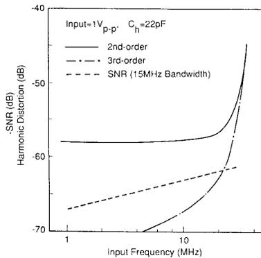
Fig. 10. Harmonic distortion and SNR frequency responses.
