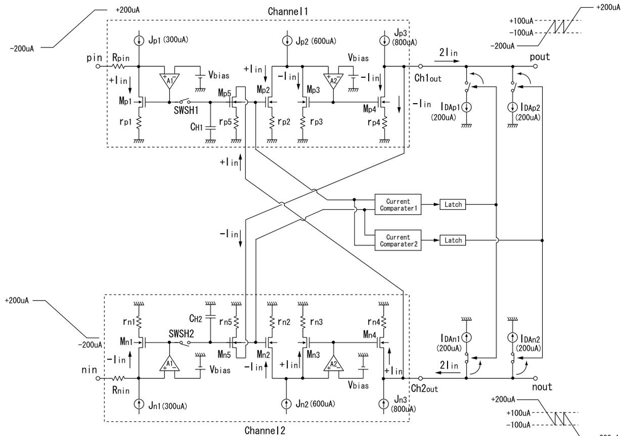
Fig. 1 The 1.5-bit bit-block circuit.
