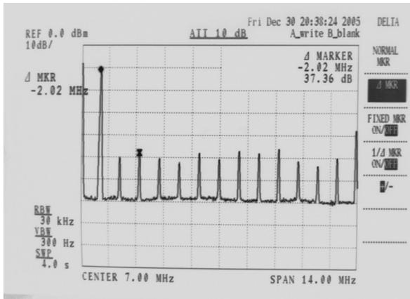
**Fig. 3** The frequency spectrum of a 1 MHz reconstructed output waveform.
