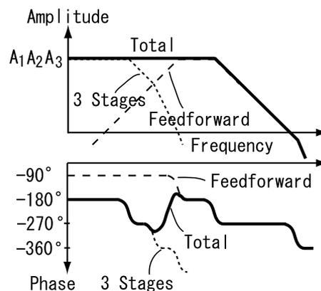
Fig. 2 Voltage gain and phase frequency characteristics of the proposed TIA.
