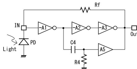
Fig. 1 Block diagram of the proposed TIA.
