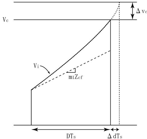
**Fig. 5** Waveforms of  $V_c$  and  $V_i$  in a current control loop (second-order slope compensation).
