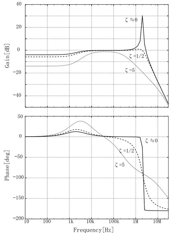
Fig. 4 Closed-loop transfer function of the current feedback loop.
