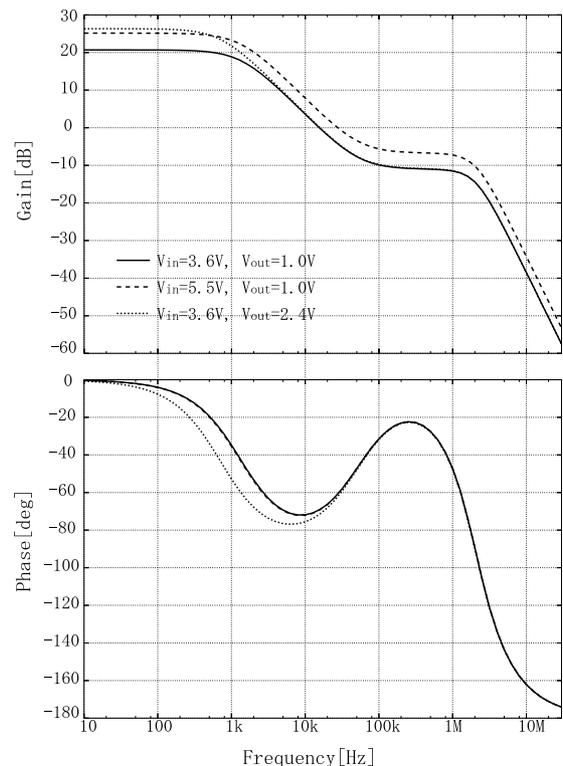
**Fig. 9** Frequency characteristics of the current feedback loop of the designed PWM buck DC-DC converter.
