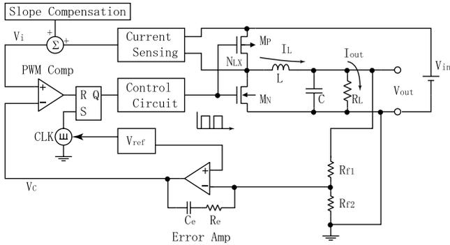
**Fig. 1** Block diagram of a PWM buck DC-DC converter with the current-mode control.
