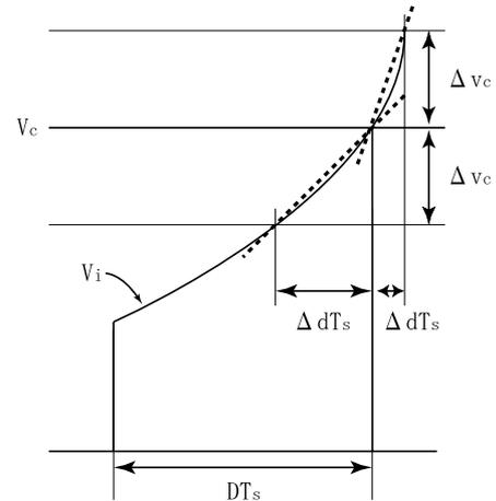
**Fig. 6** The slope necessary to perform the effective slope compensation for a large disturbance.
