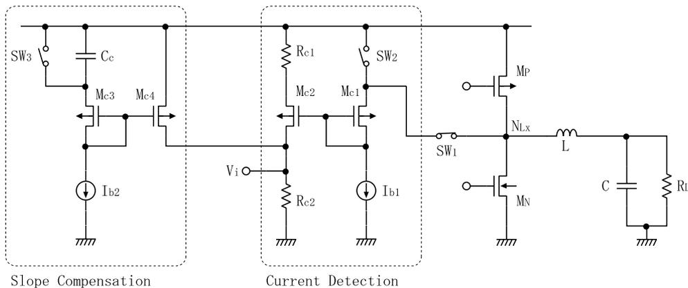
Fig. 7 Current sensing and second-order slope compensation circuit.
