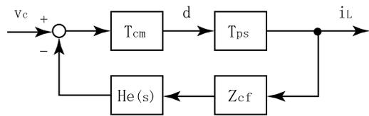
**Fig. 3** Block diagram of a current feedback control loop.
