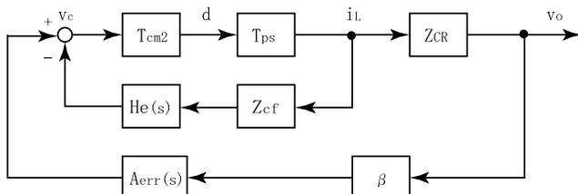
**Fig. 8** Small-signal equivalent circuit of the whole PWM buck DC-DC converter with current-mode control.
