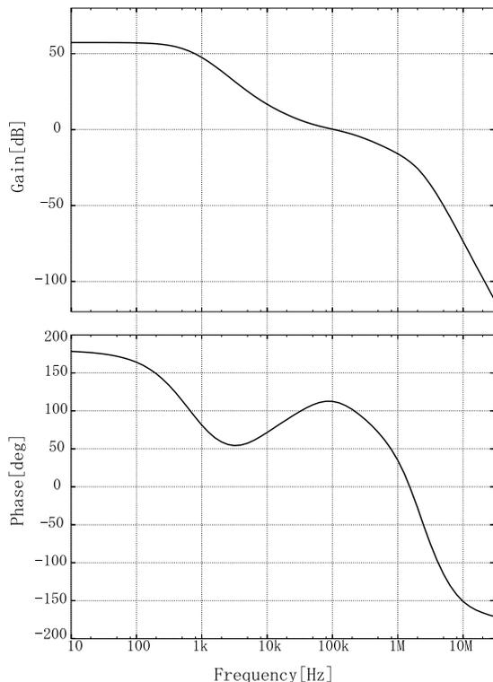
Fig. 10 Open loop transfer function characteristics of the designed PWM buck DC-DC converter with current-mode control.
