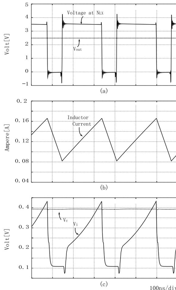
Fig. 11 The simulation result. (a) The voltage waveforms at  $N_{LX}$  and  $V_{out}$ . (b) The waveform of the current that flows through external inductor  $L$ . (c) The voltage waveforms of  $V_i$  and  $V_c$ .
