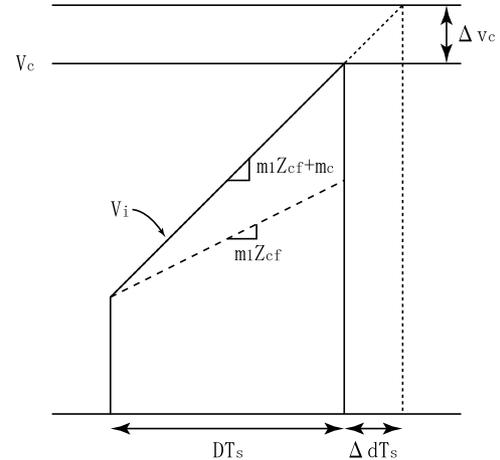
**Fig. 2** Waveforms of  $V_c$  and  $V_i$  in a current control loop.
