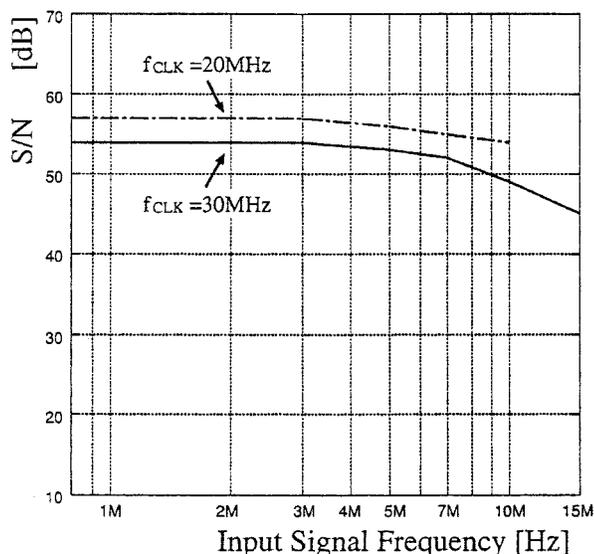
Fig. 6. Input signal frequency versus  $S/N$  characteristics (0-dB full-scale input,  $V_{cc} = 1.5$  V).
