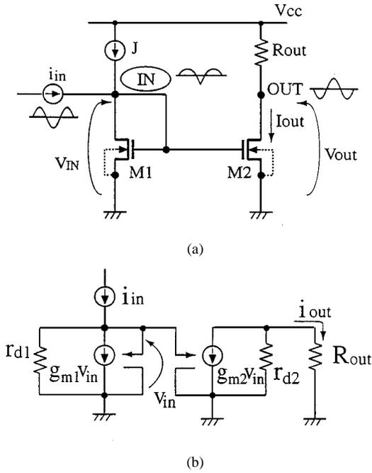
Fig. 1. (a) Conventional current-mirror circuit. (b) Small-signal equivalent circuit for input signal dependency analysis.
