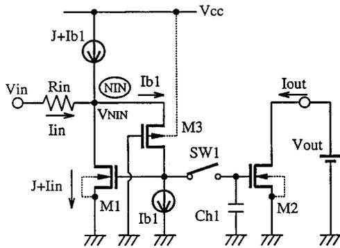
Fig. 4. High-precision low-voltage sample-and-hold circuit.
