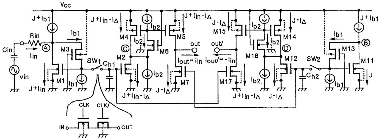
Fig. 3. Current-mode low-voltage high-performance CMOS sample-and-hold circuit.
