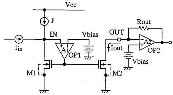
Fig. 2. High-precision current-mirror circuit.
