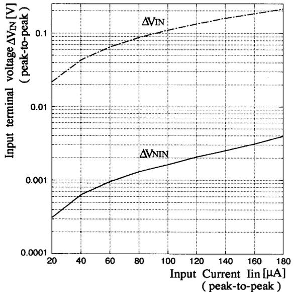
Fig. 2. Voltage change at input terminals in circuits of Fig 1(a) and (b) with various input currents.
