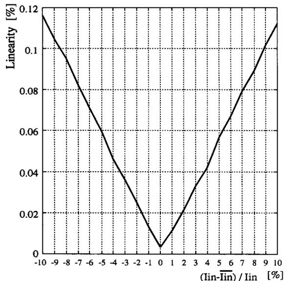
Fig. 5. Linearity degradation due to input signal unbalance.
