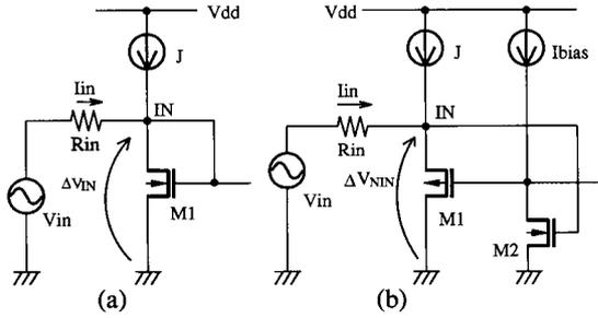
Fig. 1. Input voltage-to-current converters (a) Conventional circuit. (b) Newly developed circuit.
